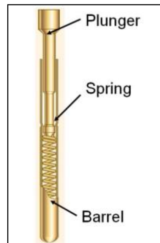
Fig. 1. Basic spring contact construction, single ended
