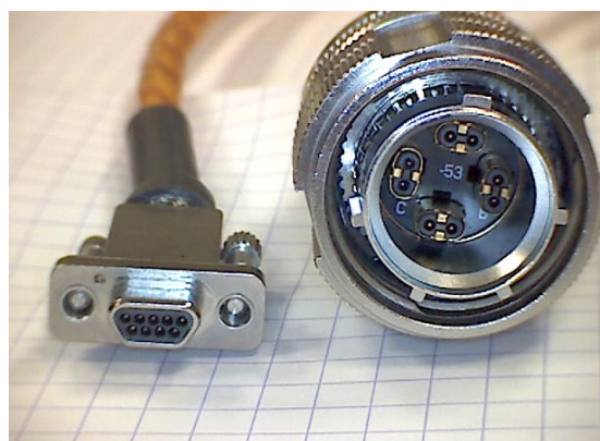
Fig.2. Comparison in size between classic 9 way Micro-D connector and one of the top HDR performers in the connector survey
