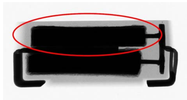
Fig. 6 Bent slugs in the same type of tantalum capacitor
