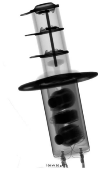
Fig. 1 X-ray view of a high voltage relay
