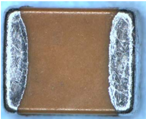
Fig. 40 Top view of failed capacitor
