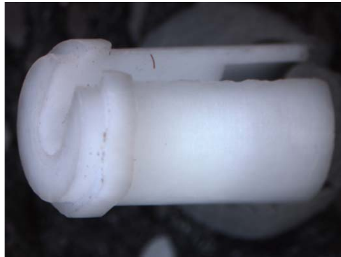
Fig. 13 The PTFE insulator exposed
