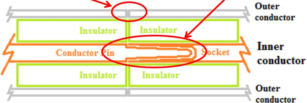
Schematic of mated RF connectors
