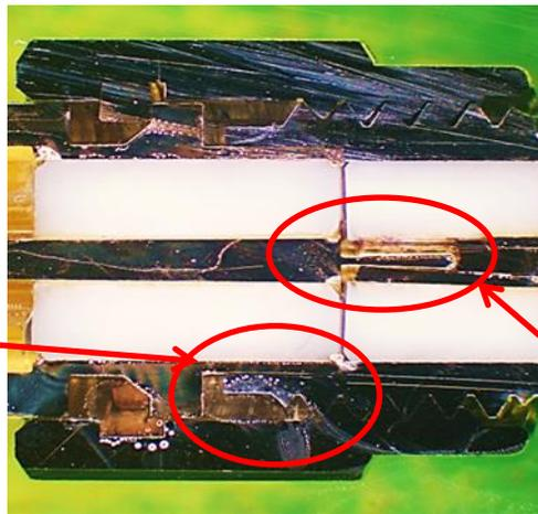
Outer RF connection, mechanically abutted and held with torqued coupling nut, no movement expected
