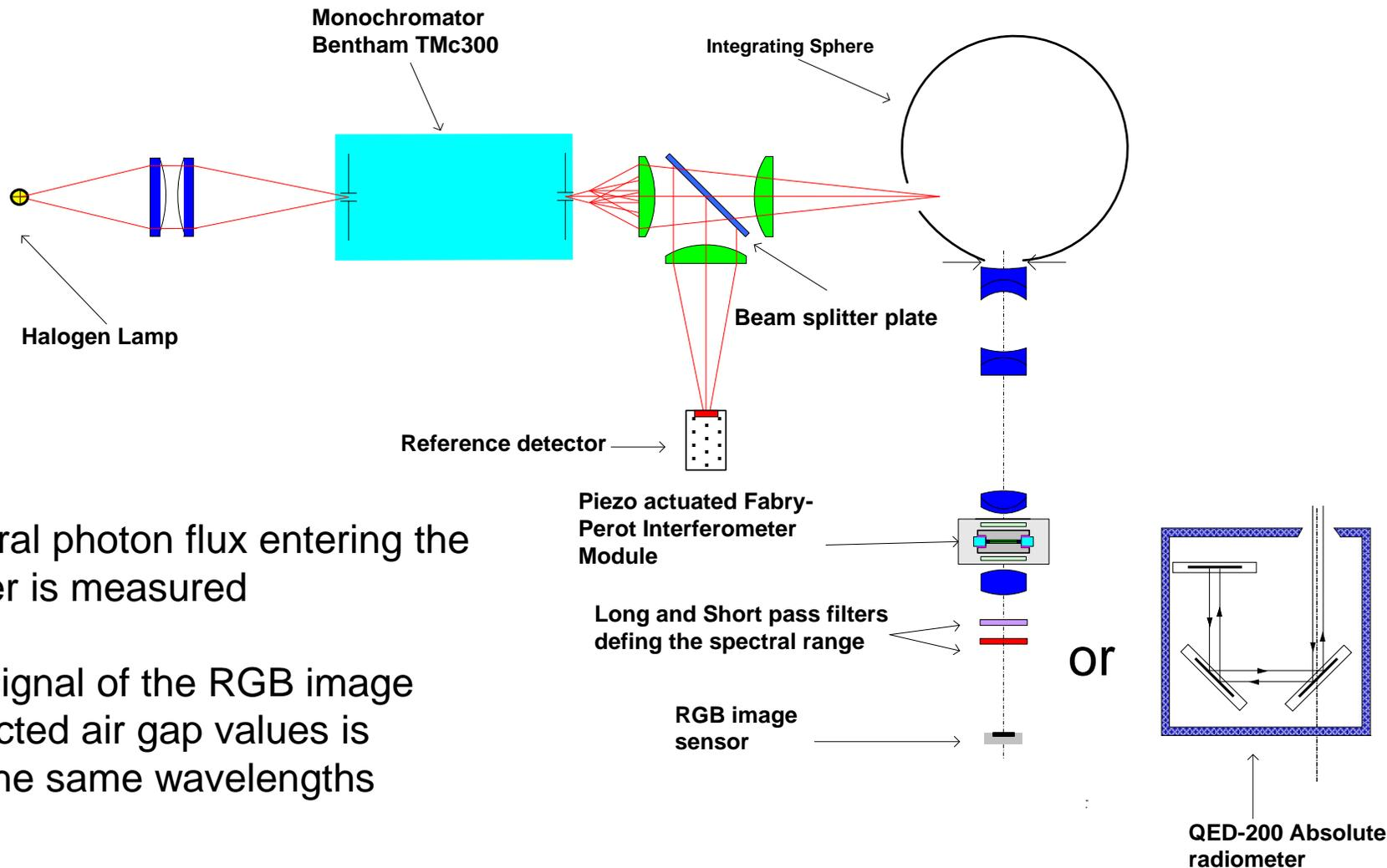
First the spectral photon flux entering the spectral imager is measured
