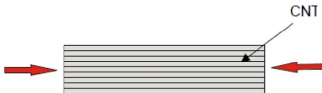
Fast-RTM-Injection: infiltration of stacked paper possible, infiltration was mainly governed by the capillary forces (Image DLR)
