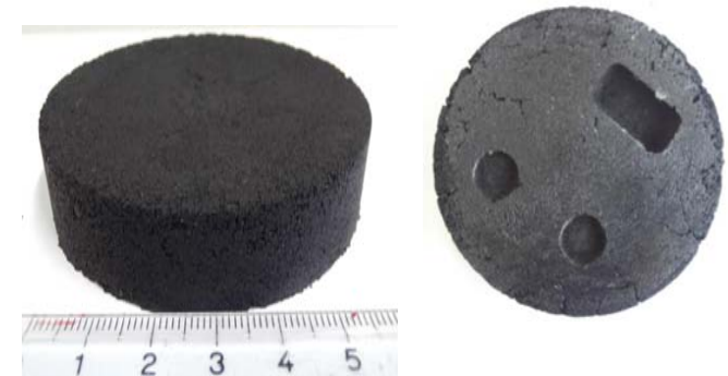
Demonstrator NACO2 Spherical upper surface different pockets by die sinking
