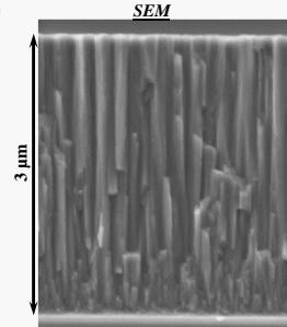
□ Synthesis of the AlTiN (+Ta, Y) by codeposition (2 targets)
