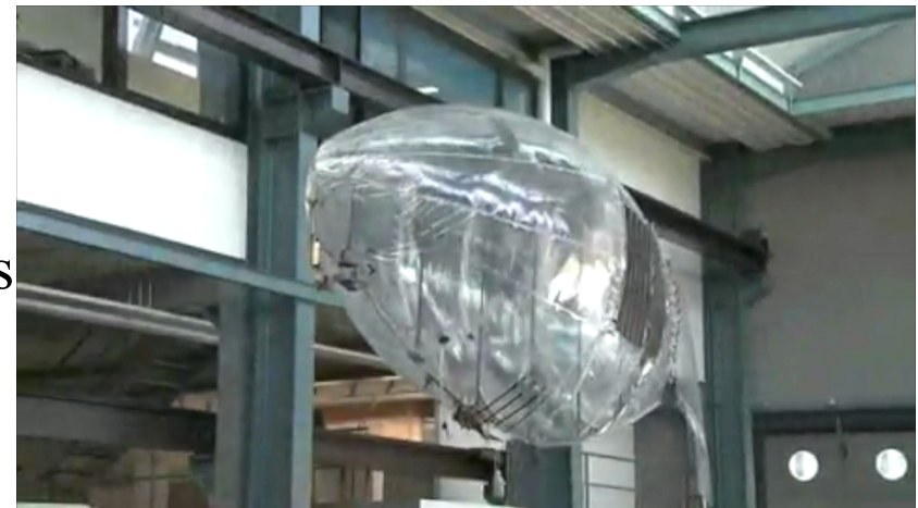
EMPA's (Zurich) 7m long blimp: "swims" through the air using 4 artificial muscles
