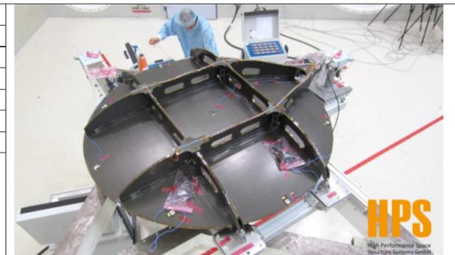
HPS full CFRP antenna reflector (project HISST2)
