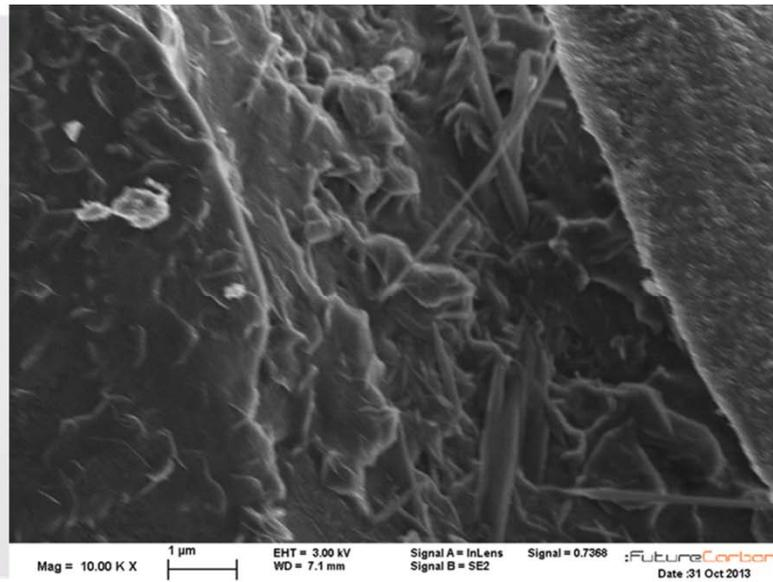
Foam route A will be used to produce larger foams; micrographs by FC; right: CNT inside the foam walls
