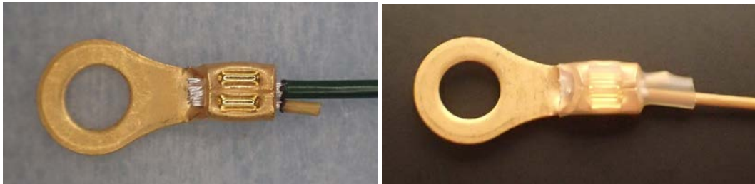
Crimping of lug with filler wire
