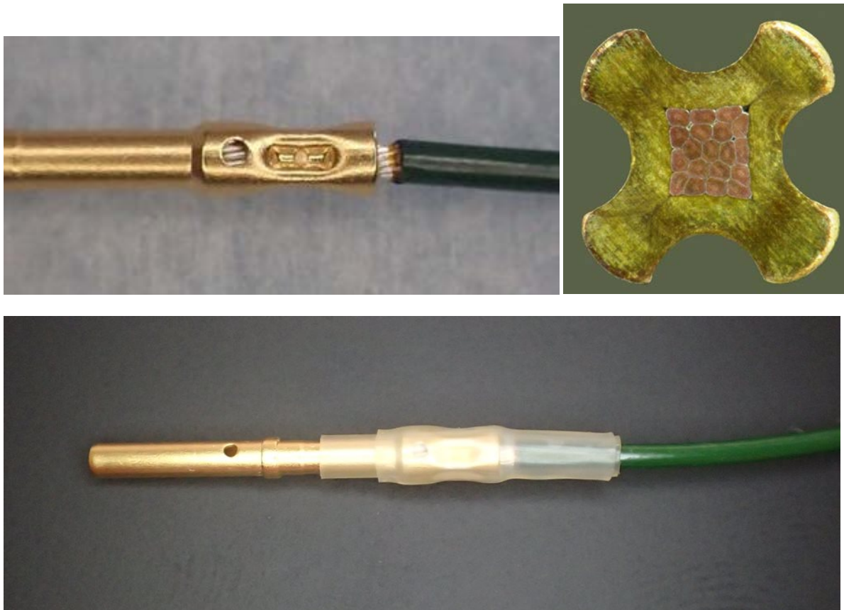
Figure 5-2: Example of a typical connector barrel and single wire crimping
