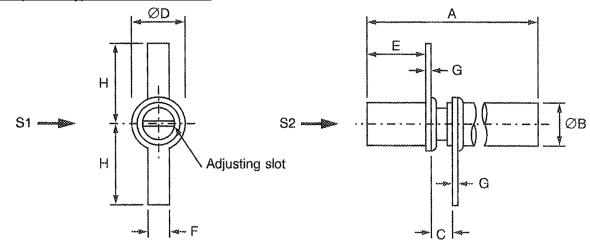
S1, S2 - Vibration and Shock axes
