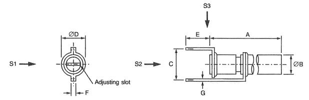
S1, S2, S3 - Vibration and Shock axes
