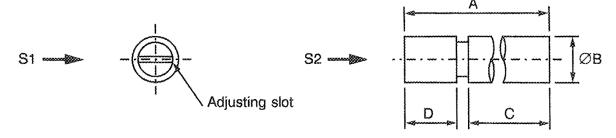
S1, S2 - Vibration and Shock axes
