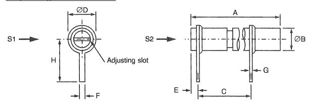
S1, S2 - Vibration and Shock axes
