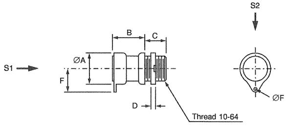
S1, S2 - Vibration and Shock axes
