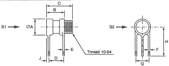
S1, S2 - Vibration and Shock axes
