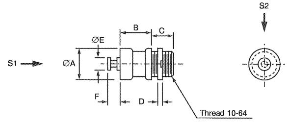
S1, S2 - Vibration and Shock axes
