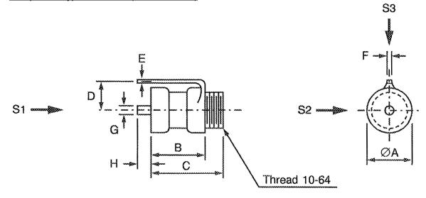
S1, S2, S3 - Vibration and Shock axes
