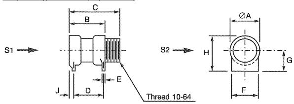
S1, S2 - Vibration and Shock axes
