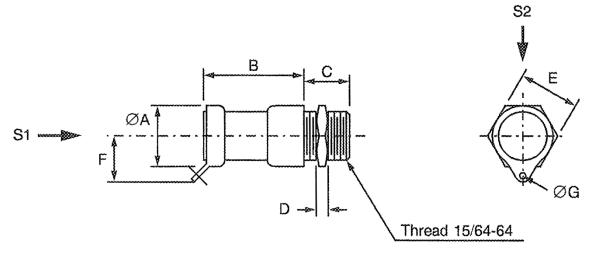
S1, S2 - Vibration and Shock axes
