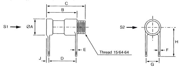
S1, S2 - Vibration and Shock axes
