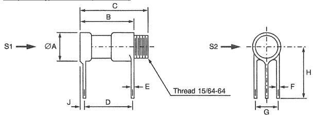
S1, S2 - Vibration and Shock axes
