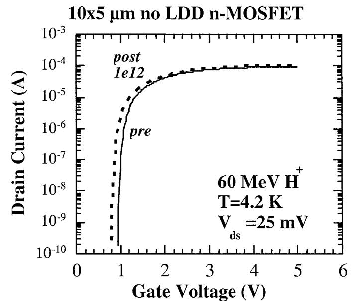
Input curves at 4.2 K and  $V_{ds}=25 \text{ mV}$  for a 10x5  $\mu\text{m}$  n-MOSFET with (left) or without (right) LDDs, corresponding to unirradiated (pre) and proton irradiated samples.
