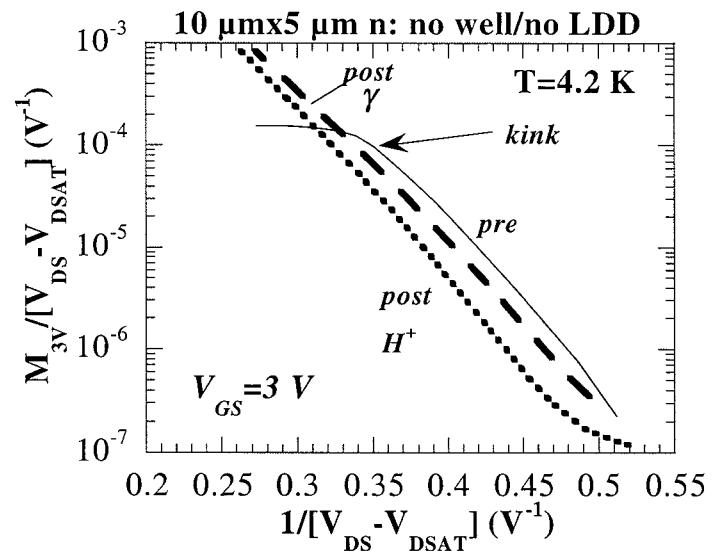
Substrate current (left) and normalised multiplication coefficient (right) for an irradiated 10  $\mu\text{m} \times 5 \mu\text{m}$  non-LDD n-MOSFET at 4.2 K.
