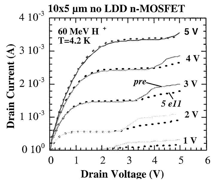
Output curves at 4.2 K and  $V_{gs}=1,2$  or 3 V for a 10x5  $\mu\text{m}$  n-MOSFET with (left) and without (right) LDDs, corresponding to unirradiated (pre) and 60 MeV proton irradiated (dashes: low-to-high; + high-to-low). No hysteresis is seen, as indicated by the arrow in the upper characteristic.
