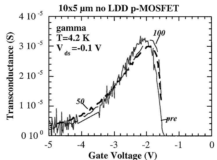
Transconductance at 4.2 K and  $V_{\text{ds}} = -0.1 \text{ mV}$  for a  $10 \times 5 \mu\text{m}$  p-MOSFET with (left) or without (right) LDDs, corresponding to unirradiated (pre) and irradiated samples (total dose).
