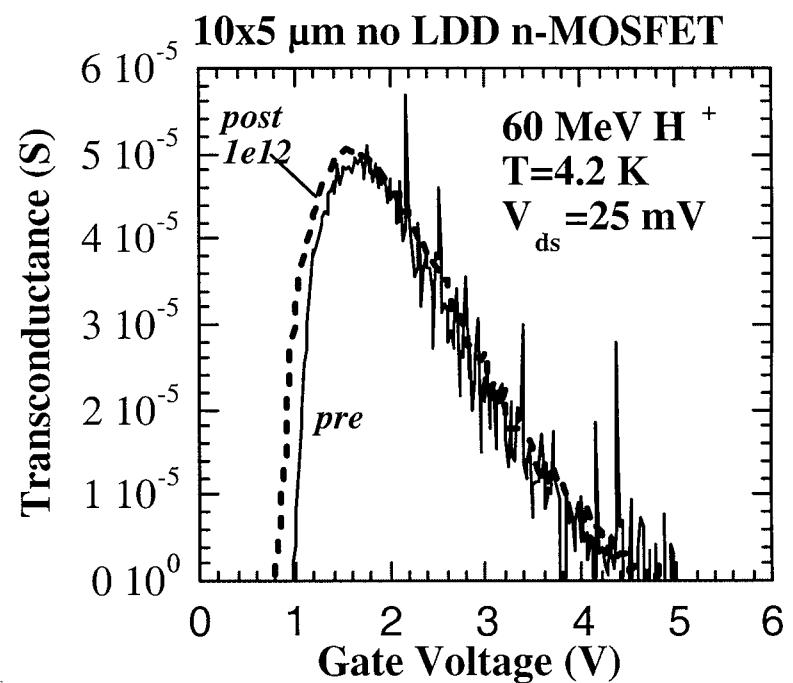
Transconductance at 4.2 K and  $V_{\text{ds}}=25 \text{ mV}$  for a  $10 \times 5 \mu\text{m}$  n-MOSFET with (left) or without (right) LDDs, corresponding to unirradiated (pre) and proton irradiated samples
