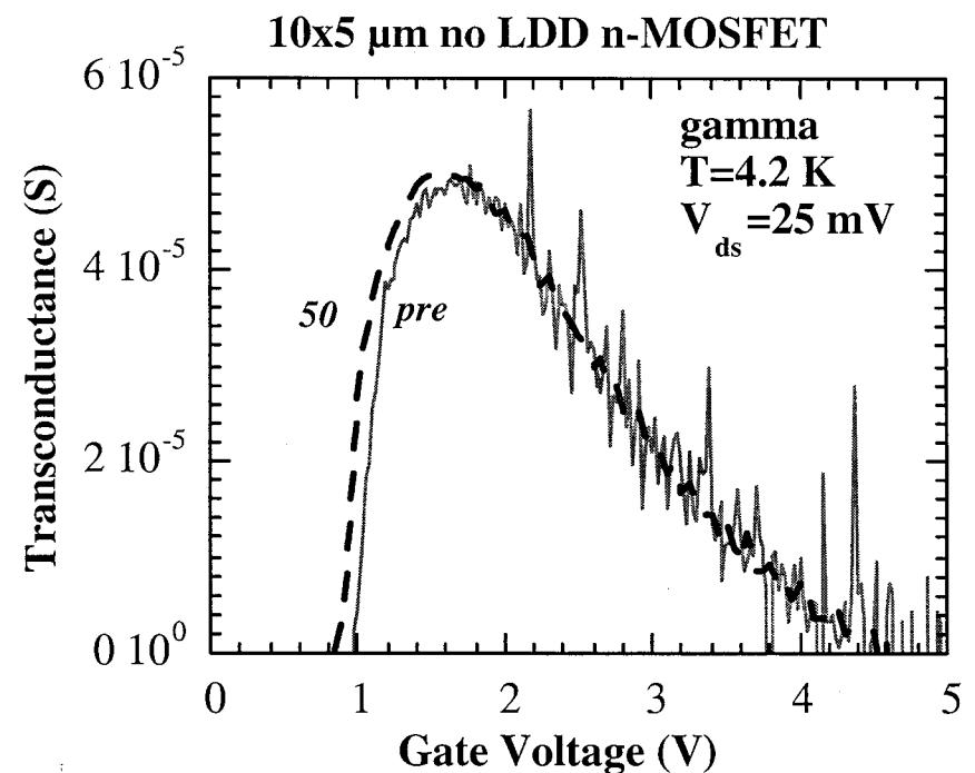
Transconductance at 4.2 K and  $V_{ds}=25 \text{ mV}$  for a  $10 \times 5 \mu\text{m}$  n-MOSFET with (left) or without (right) LDDs, corresponding to unirradiated (pre) and irradiated samples (total dose).
