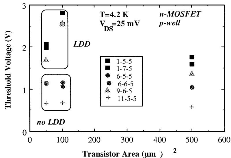
Transconductance and threshold voltage at 4.2 K for the different splits studied before irradiation.
