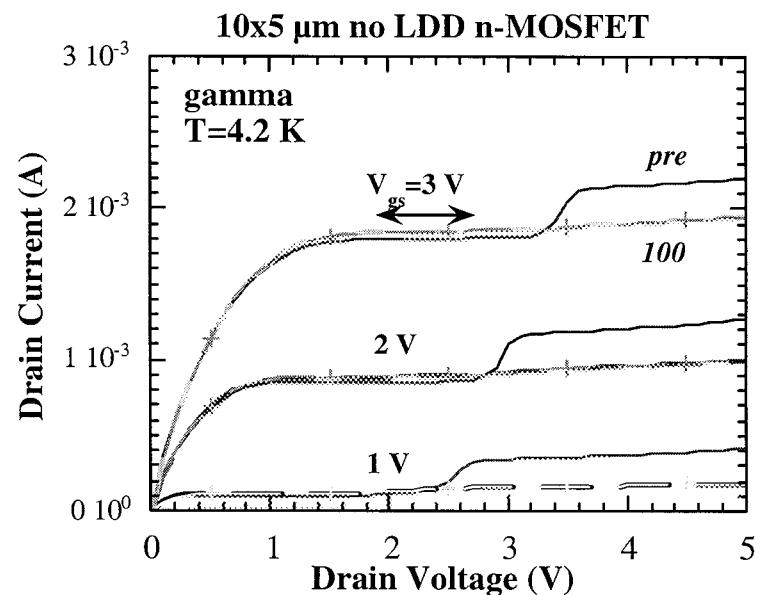
Output curves at 4.2 K and  $V_{gs}=1,2$  or 3 V for a 10x5  $\mu\text{m}$  n-MOSFET with (left) and without (right) LDDs, corresponding to unirradiated (pre) and 100 krad(Si) (dashes: low-to-high; + high-to-low). No hysteresis is seen, as indicated by the arrow in the upper characteristic.
