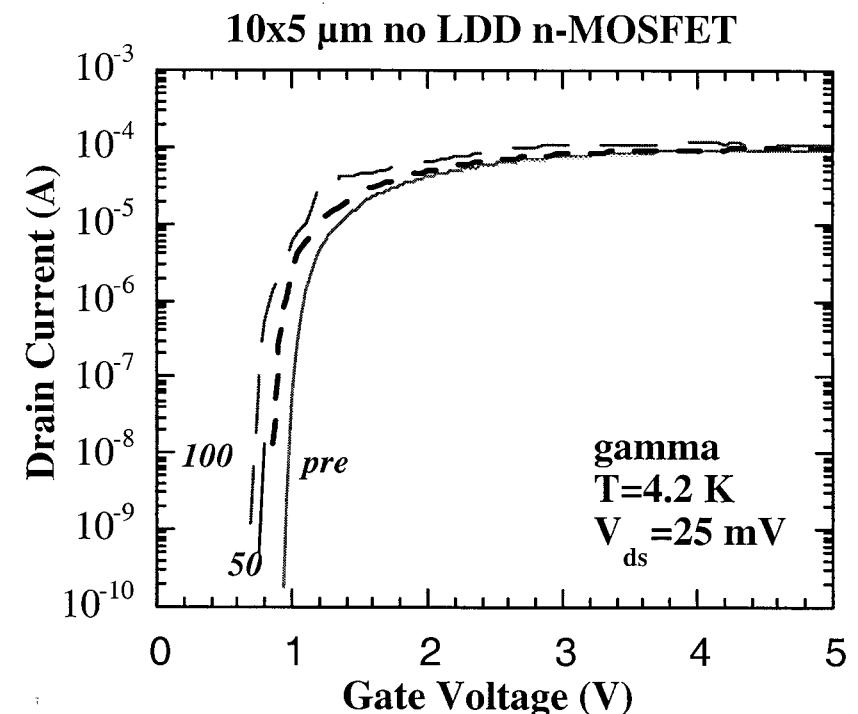
Input curves at 4.2 K and  $V_{ds}=25 \text{ mV}$  for a 10x5  $\mu\text{m}$  n-MOSFET with (left) and without (right) LDDs, corresponding to unirradiated (pre) and irradiated samples (total dose).
