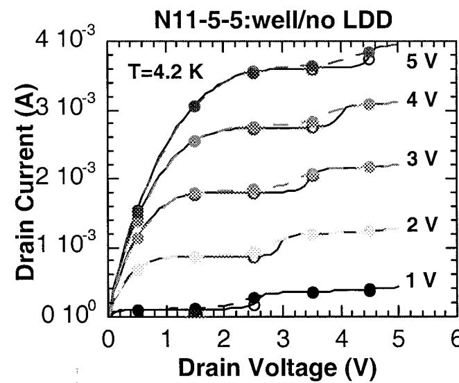
$I_d - V_{ds}$  at 4.2 K and  $V_{ds}=25$  mV for different geometry n-MOSFETs with (left) and without (right) LDDs, before irradiation.
