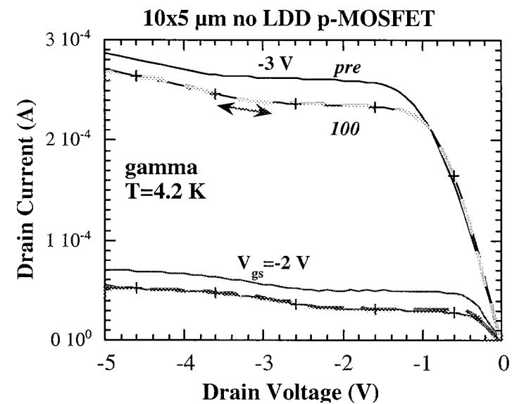
Output curves at 4.2 K and  $V_{gs} = -2$  or  $-3$  V for a  $10 \times 5 \mu\text{m}$  p-MOSFET with (left) and without (right) LDDs, corresponding to unirradiated (pre) and 100 krad(Si) (dashes: low-to-high; + high-to-low). No hysteresis is seen, as indicated by the arrow in the upper characteristic.
