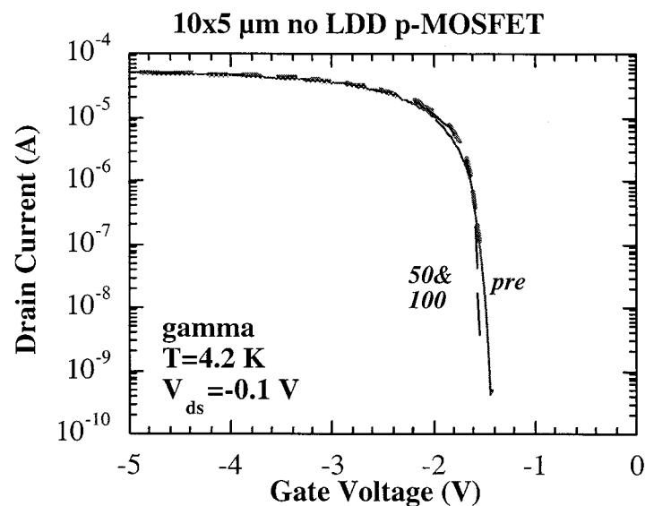
Input curves at 4.2 K and  $V_{ds} = -0.1 \text{ mV}$  for a  $10 \times 5 \mu\text{m}$  p-MOSFET with (left) or without (right) LDDs, corresponding to unirradiated (pre) and irradiated samples (total dose).
