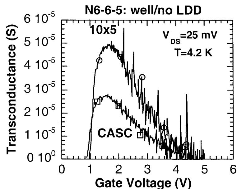
Transconductance at 4.2 K and  $V_{ds}=25 \text{ mV}$  for different geometry n-MOSFETs with (left) and without (right) LDDs, before irradiation.
