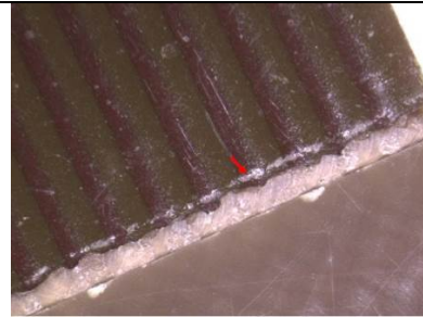
Figure 10-84: Example of an acceptable superficial scratch
