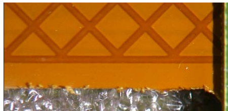
Figure 10-86: Examples of burrs on edge of flex
