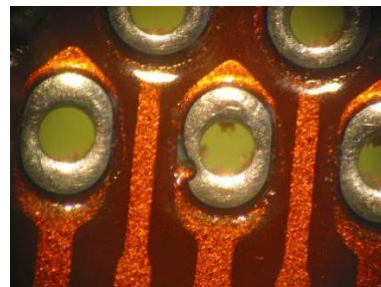
Figure 10-101: Pad diameter reduction due to local coverage by coverlay or resin squeeze out
