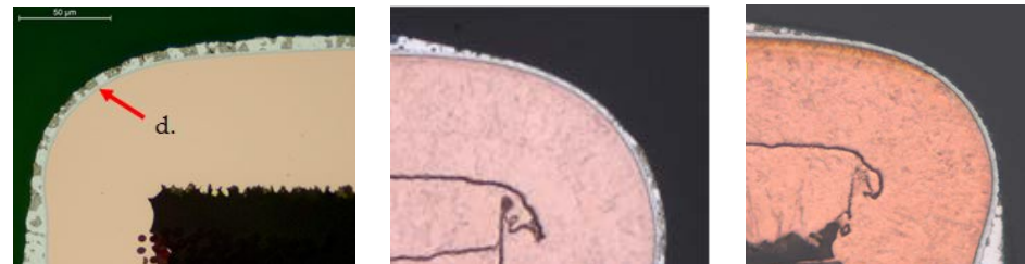
Figure 10-22: Tin-lead thickness on PTH corner – target thickness (left), coverage of less than 1 µm (middle), absence of SnPb on IMC (right)
