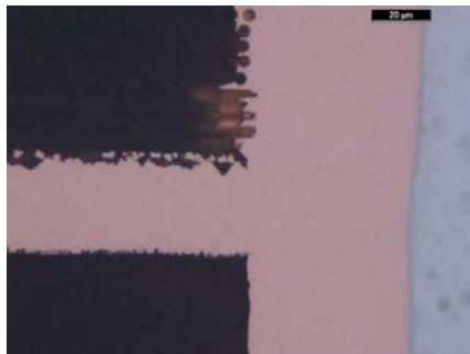
Figure 10-51: Interconnect after stress, target condition, after microetch (top) and as-polished (bottom)
