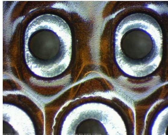
Figure 10-94: Hole misregistration causing reduced annular ring
