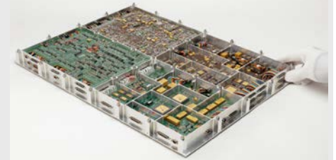
Mars Rover on-board computer
