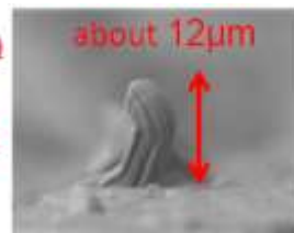
Ground (1 st year) 5750 size chip capacitor (C31) Electrode plating part
