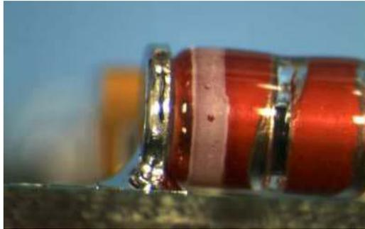
Figure I-9: Acceptable, terminal wetted along end, face and sides (see also Table 11-1)
