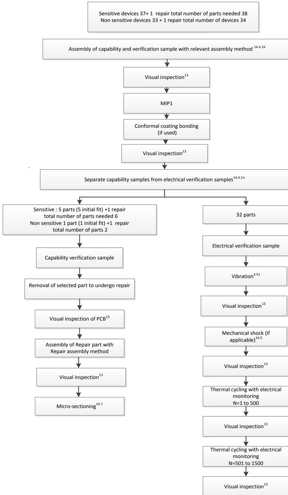
**Figure 14-2: Verification programme flow chart (electrical testing)**
