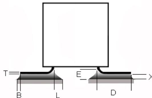
**Figure 11-13: Mounting of stacked modules devices with leads protruding vertically from bottom**
