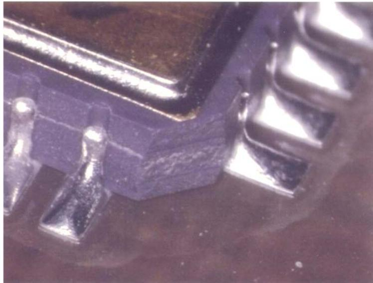
**Figure I-24: LCC General view, acceptable solder joints**
