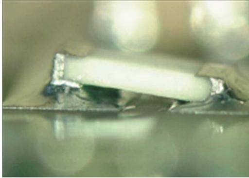
**Figure I-6: Unacceptable, excessive tilt (see also Table 11-1)**
