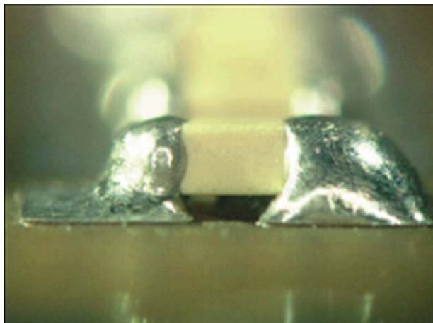
**Figure I-4: Unacceptable, excessive solder (see also Table 11-1)**
