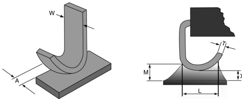
**Figure 11-7: Mounting of devices with “J” leads**
