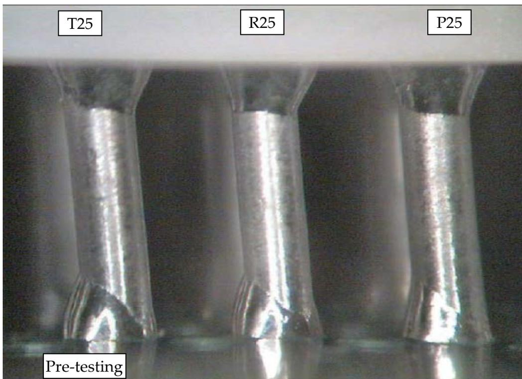
NOTE: Asymmetry of solder fillets at PCB is consequence of teardrop footprints and is acceptable
