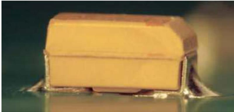
**Figure I-23: Acceptable, preferred solder joint**
