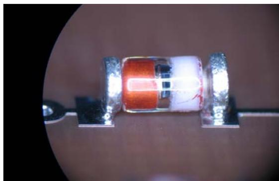
Figure I-12: Unacceptable overhang
