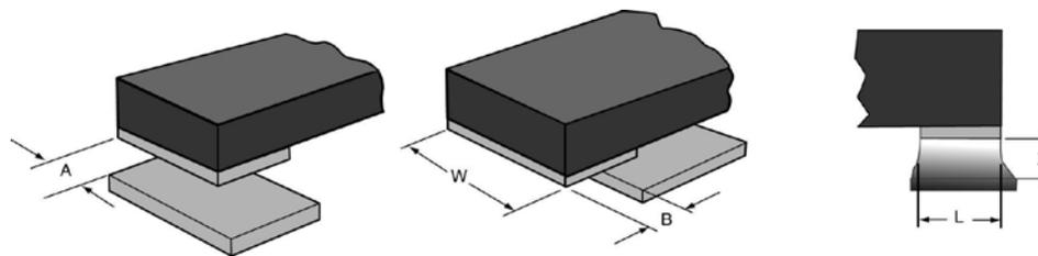
**Figure 11-2: Mounting of bottom terminated chip devices**
