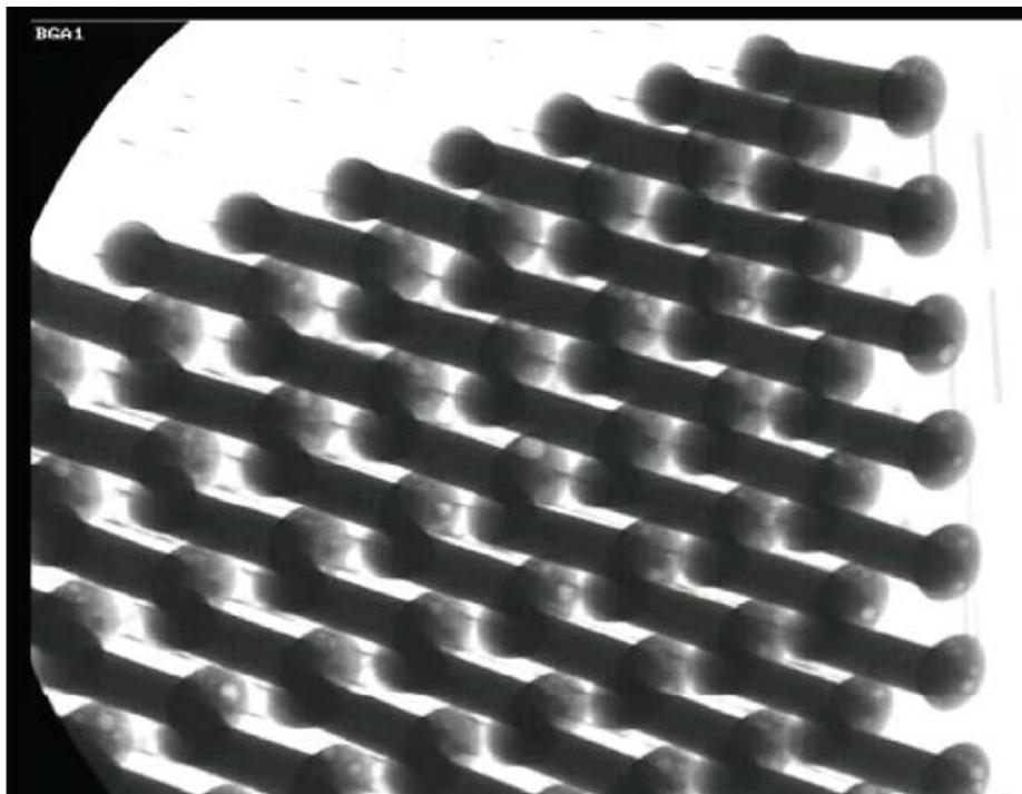
Figure I-33: X-radiograph of CGA showing solder fillets at base of columns:
