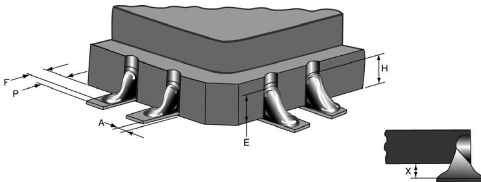
**Figure 11-5: Mounting of castellated chip carrier devices**
