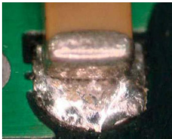
**Figure I-5: Unacceptable, poor wetting (see also Table 11-1)**
