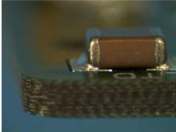
**Figure I-3: Acceptable, minimum Solder (see also Table 11-1)**
