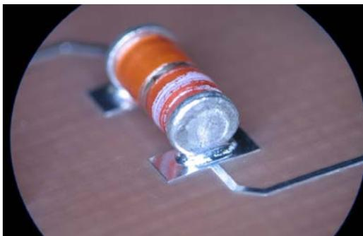
Figure I-11: Not Acceptable, insufficient solder joint (see also Table 11-3)
