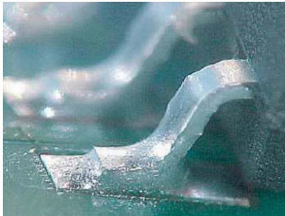
**Figure I-14: Examples of gull-wing device with rectangular lead: Acceptable**
