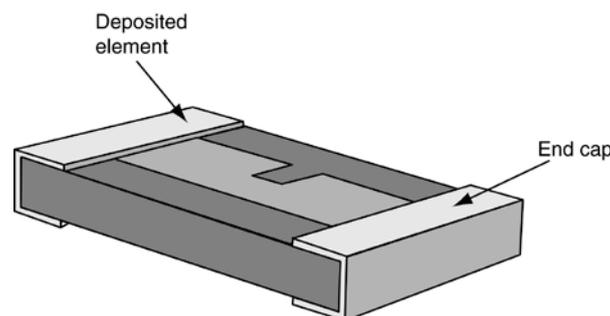
Figure 9-1: Exposed element
