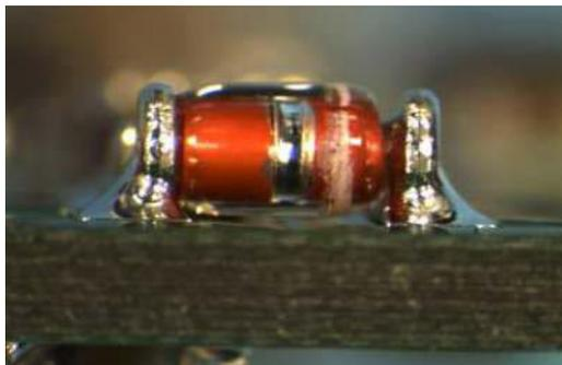
Figure I-10: Acceptable, maximum solder joint (see also Table 11-3)
