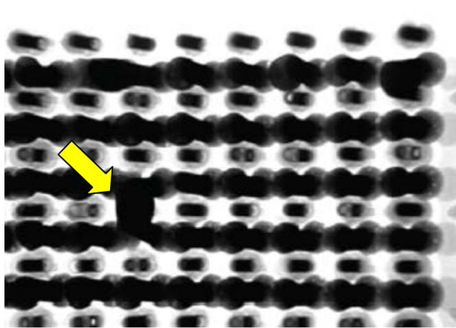
Figure I-32: X-radiograph of CGA mounted on PCB showing solder bridge: Reject
