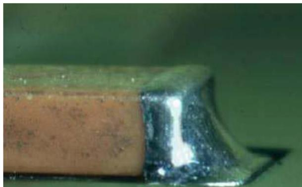
**Figure I-2: Acceptable, maximum solder (see also Table 11-1)**
