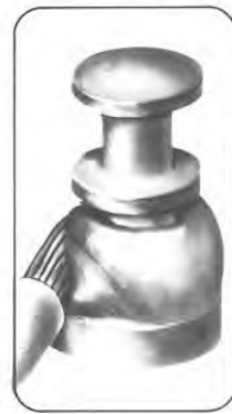
Unacceptable Excessive solder
