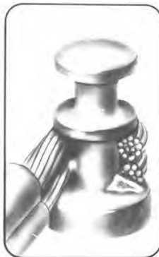
Unacceptable Insufficient solder
