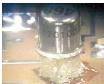
Figure 8-2: Staking of TO package with underfill
