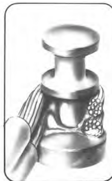
Acceptable Minimum solder
