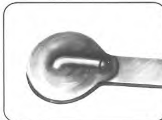
Acceptable Minimum solder
