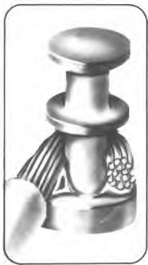
Unacceptable Insufficient solder
