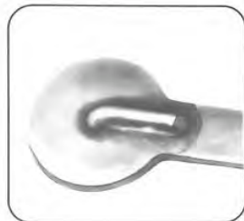
Unacceptable Insufficient solder
