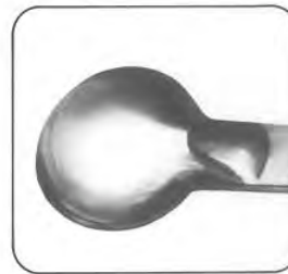
Unacceptable Excessive solder
