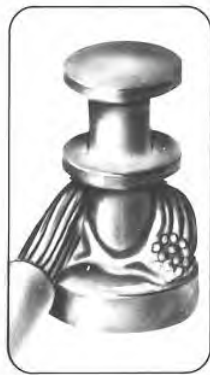
Acceptable Minimum solder
