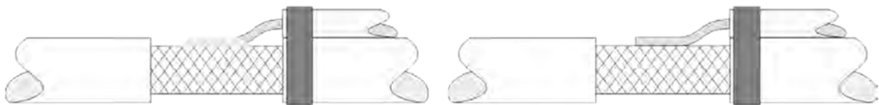
(b) Securing with shrink sleeving
