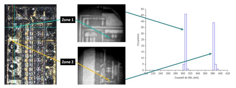
Laser test Pulse energy = 2.1nJVCC = 5VT =  $125^{\circ}C$
