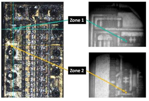
Test procedure : 100 SEL (50 per sensitive zone) over 5 devices
