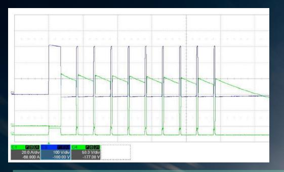
Trr<10ns Vrev = 300V Surge current I=64A flattens out to an Iavg=40A for 100µs every 20ms duty cycle = 0.005
