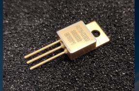
A new heavy ions test with representative GALA conditions were performed by Alter : Vr max was increased to 360V, LET=46.1MeVcm2/mg, Fluence up to e+6 p/cm2 DUTs were submitted to HTRB after irradiation
