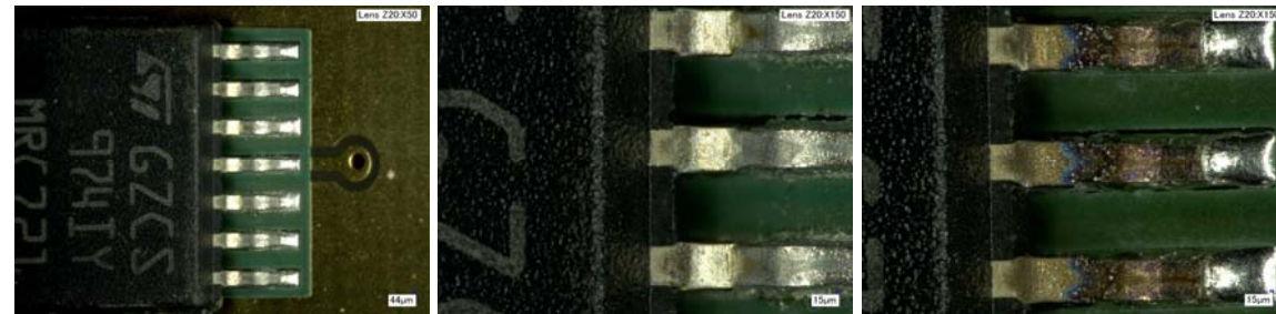
Post Stress High Magnification Inspection – No Sn Whisker Growth Evident
