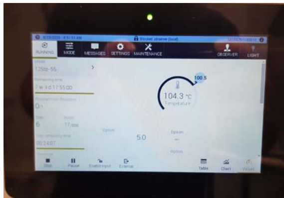
Capacitor TC Test Vötsch LabEvent T40/70/5 Single Chamber System
