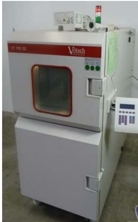
Active Component TC Test Vötsch VT7012/S2 Dual Chamber System
