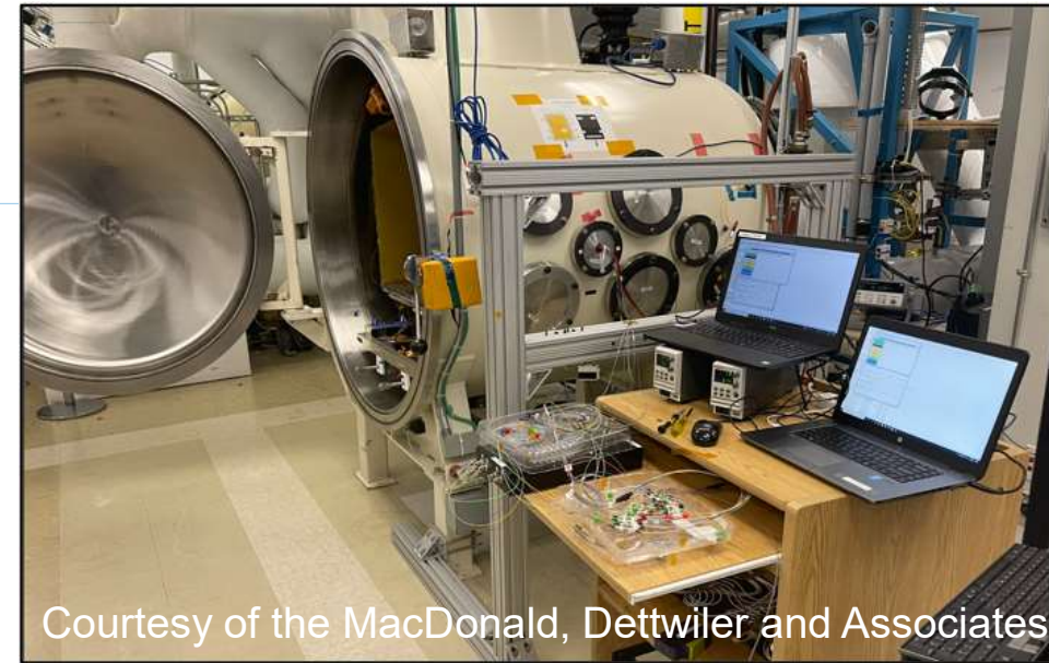
Figure 11. TVAC Testing Chamber and Test Station
