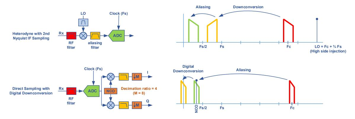
Benefit of architecture based on Direct Sampling with Digital Down Sampling over Heterodyne architecture is more flexibility when selecting frequency bands.
