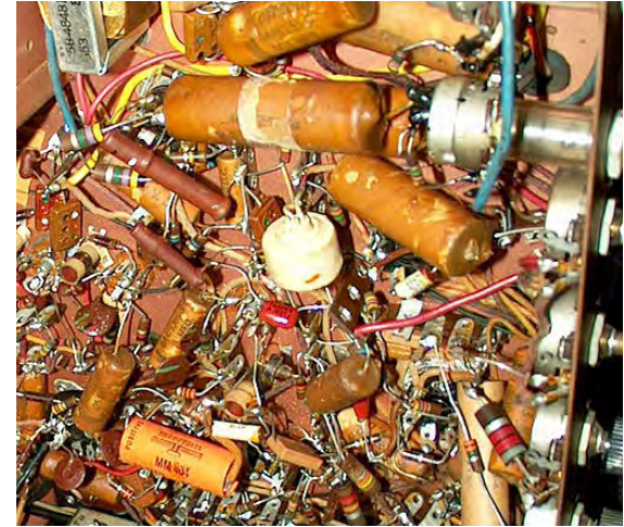
1948 Motorola TV ↑ point-to-point wiring ↓
