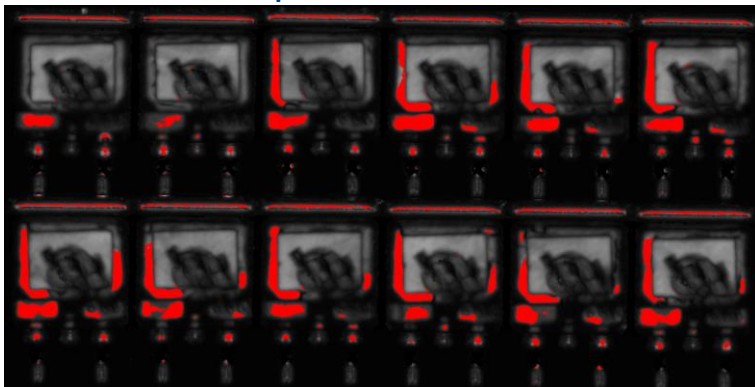
No significant evolution of delamination after 100 cycles
