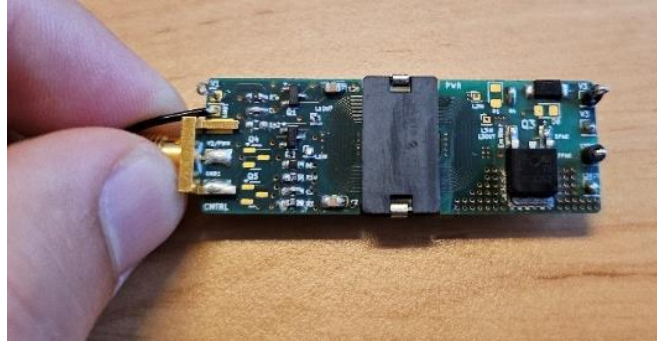
Second tested prototype (integrated planar transformer)
