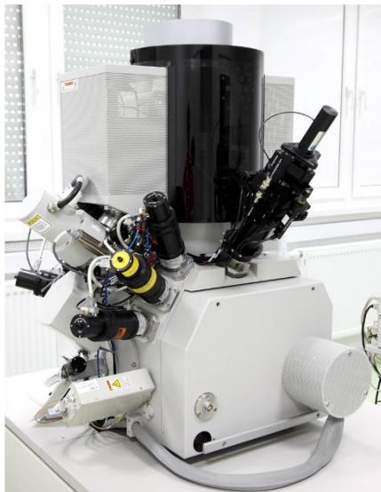
SEM/FIB system - Helios NanoLab 600 DualBeam
