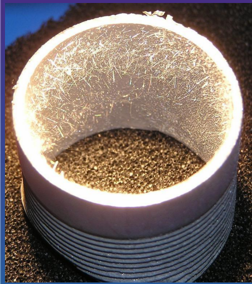
Zinc whiskers on steel pipe [1]
