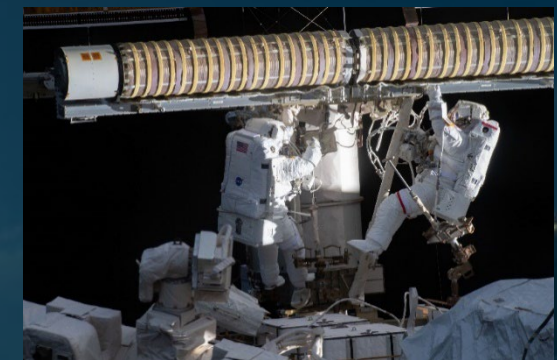
Installation of roll-out solar arrays on the ISS - ©NASA/ESA
