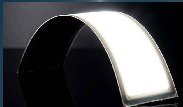
Flexible white OLEDs for solid-state lighting. © OLEDWorks
