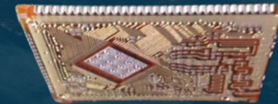
Side mounting on PCBs, created by Nano Dimension DragonFly Pro
