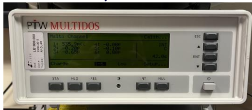
Electrometer: Live monitoring of charge
