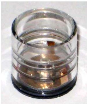
Figure 12 - Engineering model of the glass tube including valve and nozzle
