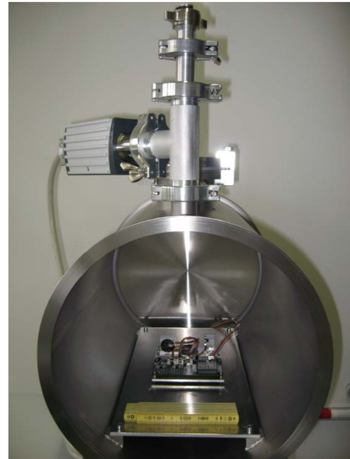
Engineering model of the micro wheel system in vacuum chamber at TU Berlin
