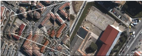
A high-resolution remote sensing camera featuring a novel prism structure with several CCDs creating an image mosaic of 10200 x 1600 pixels. The image is taken from the Barcelona area.
