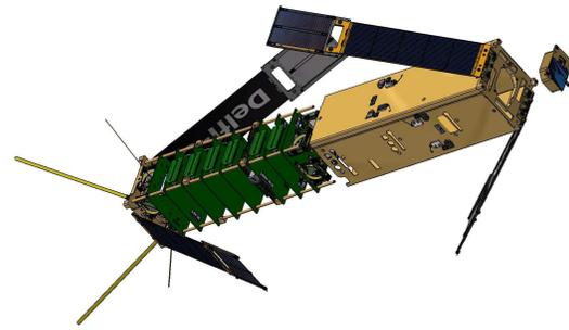
**Fig. 4** Exploded view of the Delfi-C<sup>3</sup> three-unit CubeSat of the Delft University of Technology.
