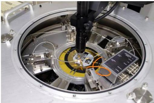
Figure 3 Fully automated ELT, C-V and stepping procedures within a controlled atmosphere chamber(PAV150, Suss MircoTec)
