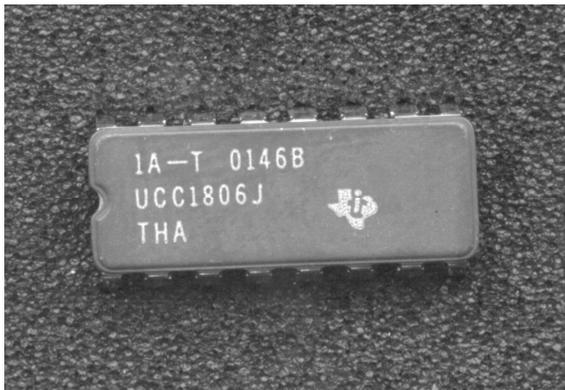
Figure 3.1.1 Package, top view
