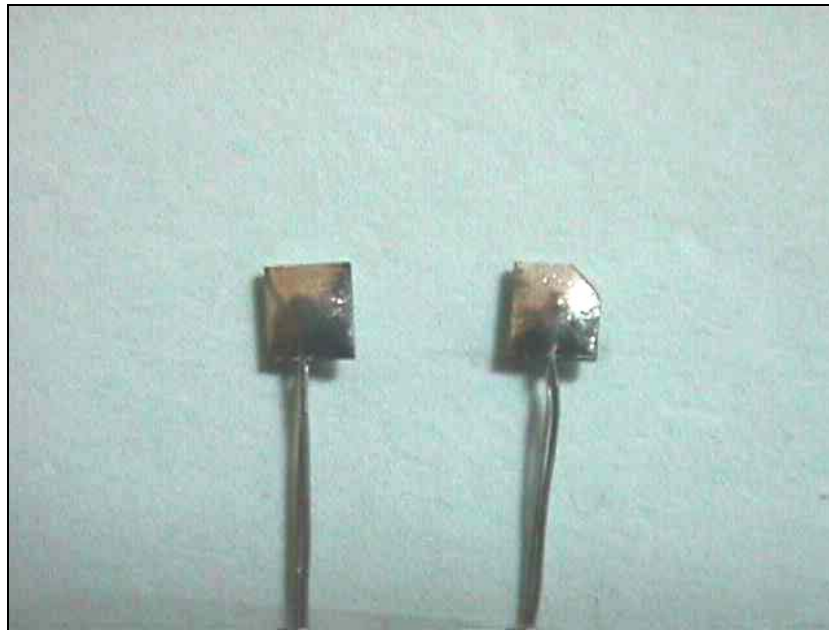
Figure 1.4.2 – Component before and after abrasion resistance adjustment
