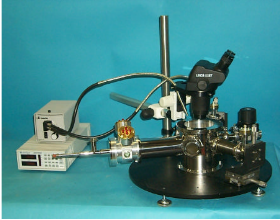
Figure 3: Picture of the Janis cryostat that is used for the cryogenic irradiation.
