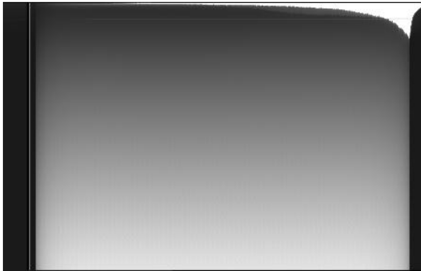
Figure 5.5.4-1 Dark image at 24.9°C from CCD#1 after 17.9 krad(Si) cobalt60 irradiation
