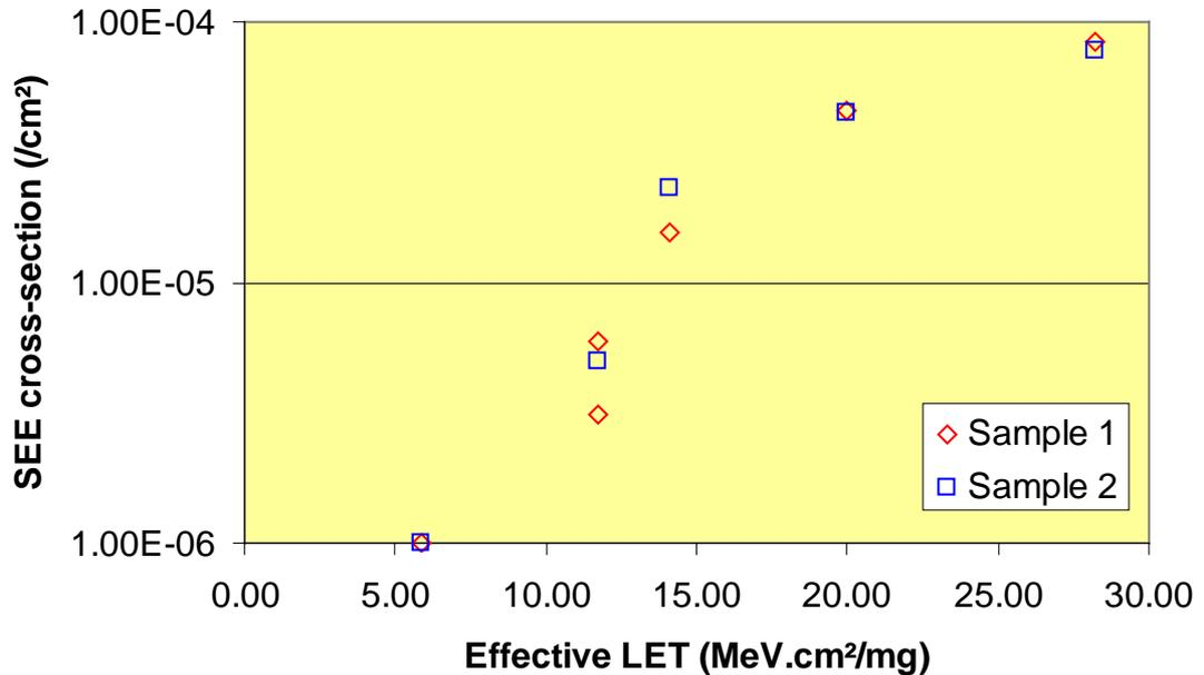
Figure 3 – ATF22V10C SEE error cross-section versus LET
