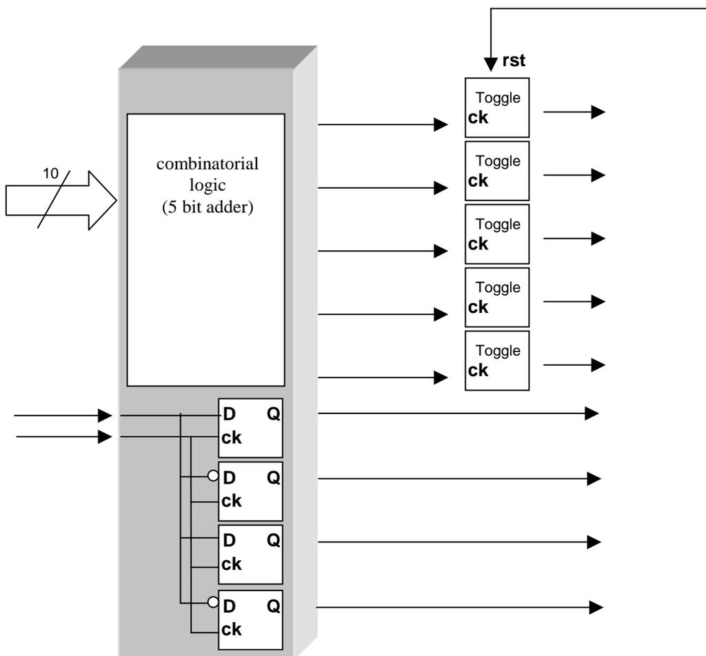
Figure 2 – Test principle
