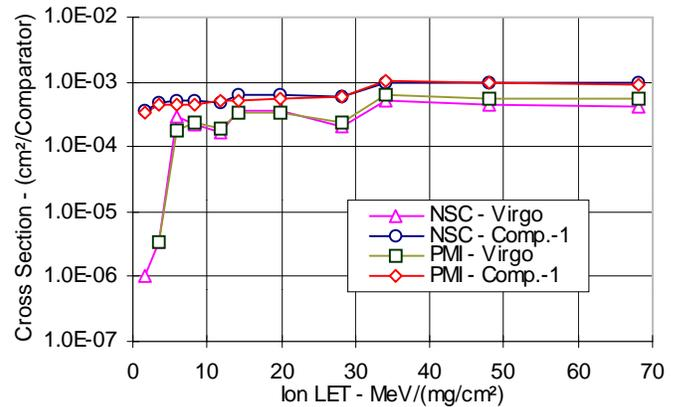
Fig. 3. NSC LM139J and AD/PMI PM139 Heavy ion SET results – VIRGO and Comparator tested.
