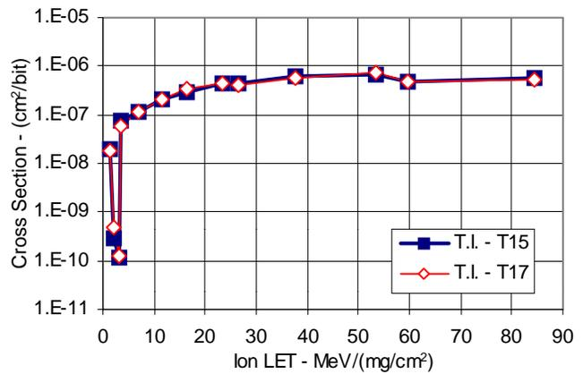
Fig. 6. T.I. SMX44100-80 4Mx1 DRAM Rev. B S2.1. – Heavy ion SEU results
