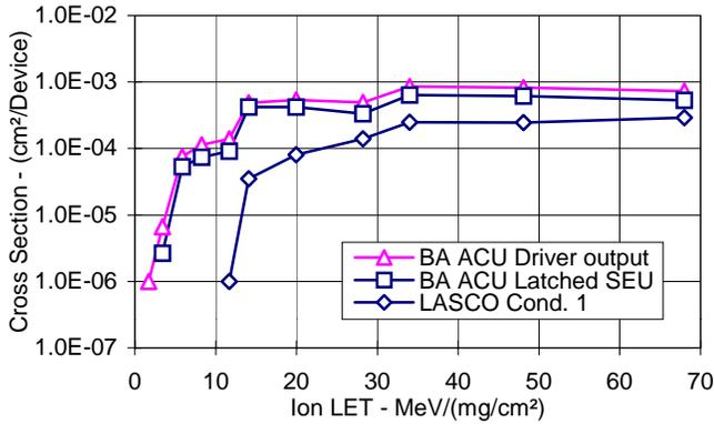
Fig. 5. Unित्रode UC1707J Heavy ion SET results – BA ACU and LASCO tested.
