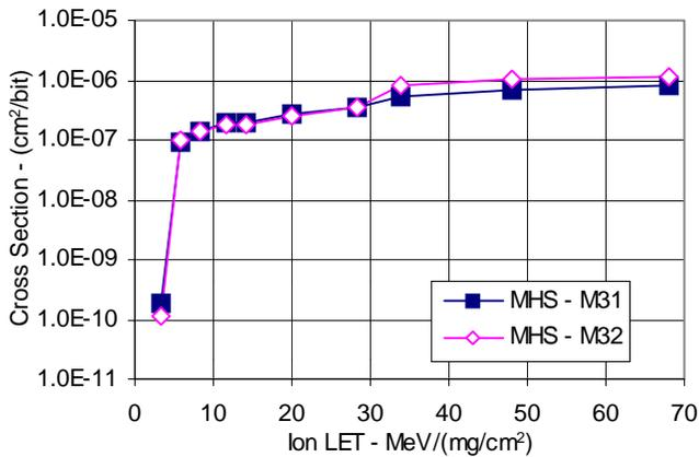
Fig. 8. MHS CP65656EV 32K8 SRAM – Heavy ion SEU results
