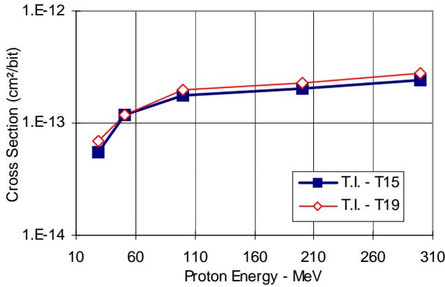
Fig. 7. T.I. SMX44100-80 4Mx1 DRAM Rev. B S2.1. – Proton SEU results
