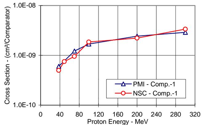
Fig. 4. NSC LM139J and AD/PMI PM139 Proton SET results – Comparator 1 tested.
