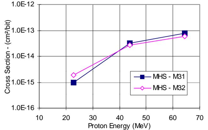
Fig. 9. MHS CP65656EV 32K8 SRAM – Proton SEU results
