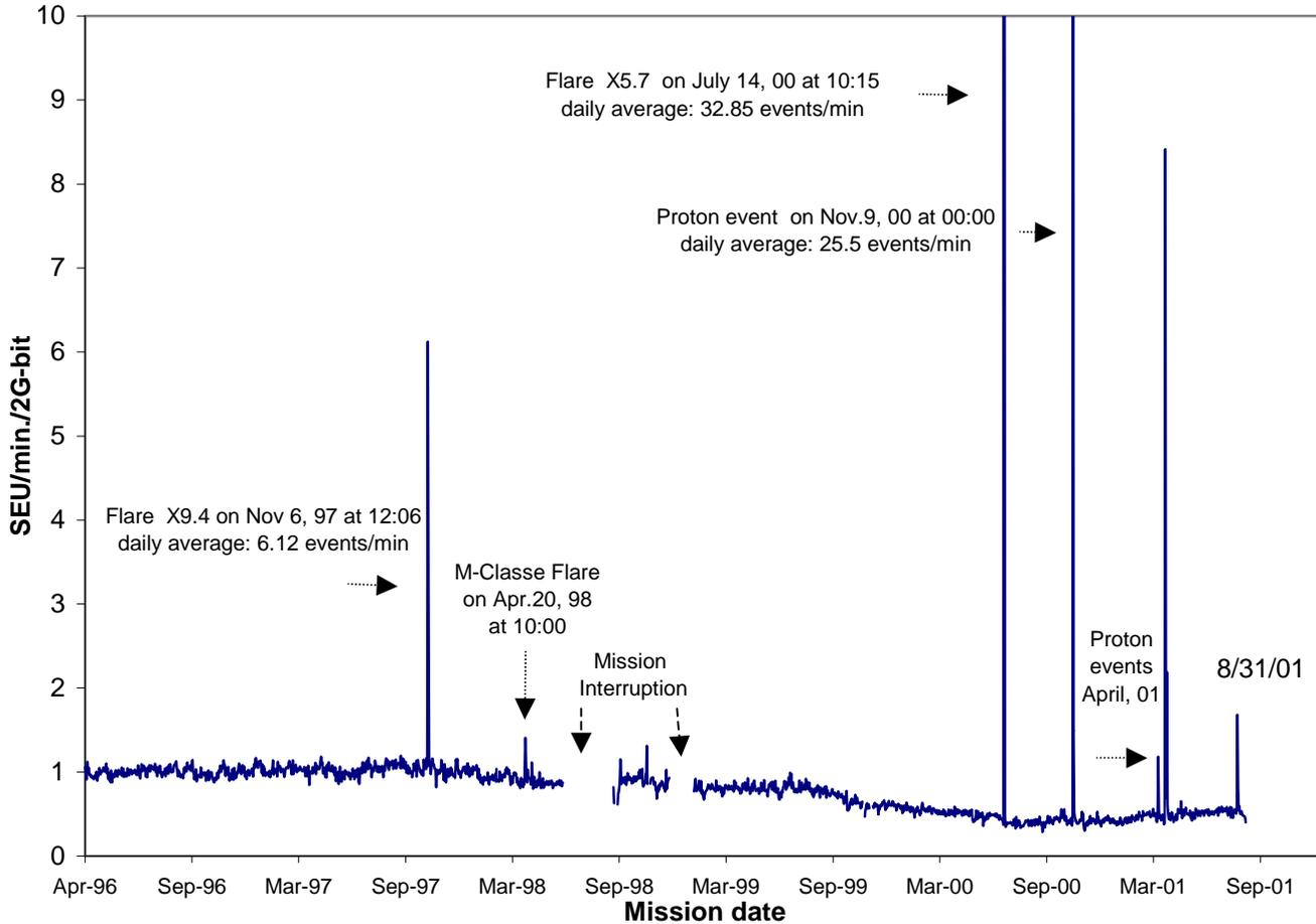
Fig. 1. SEU upset rate for 2 G-bit T.I. 4Mx1 DRAMs.
